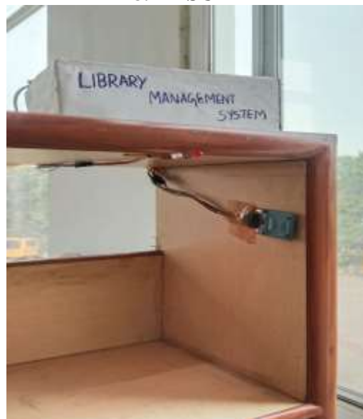
Fig 6: Implementation of RFID based book shelving system in library
